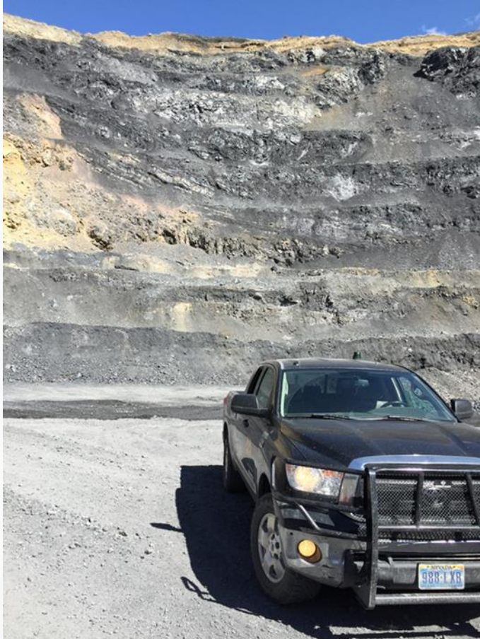
Open pit benches with exposed mineralization
